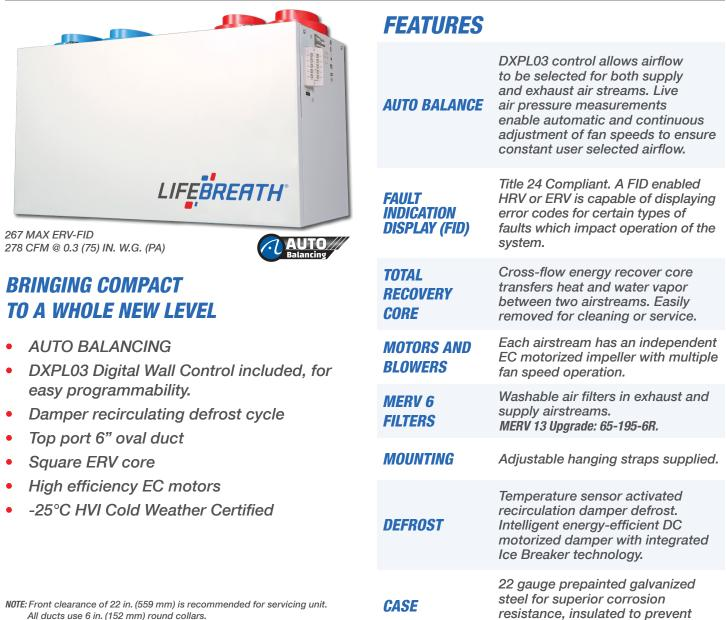
All ducts use 6 in. (152 mm) round collars. All units conform to CSA and UL standards.
