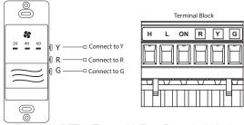
Figure 34. DET01 Timer with Type B terminal block
