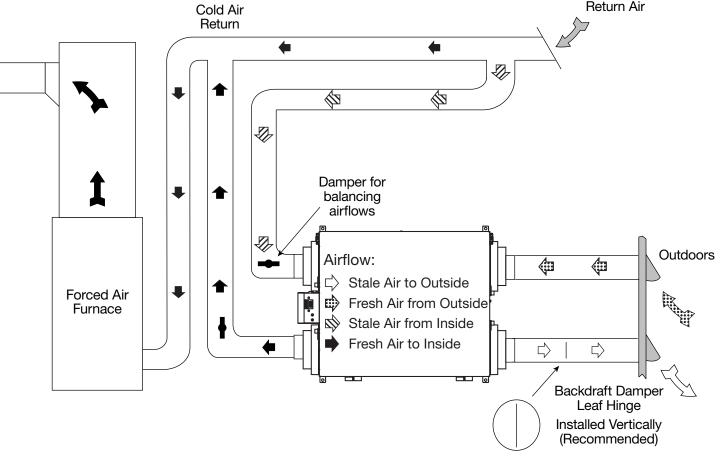
Figure 18. Simplified Installation (Return/Return)
