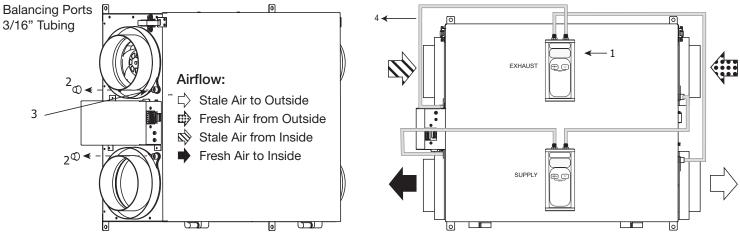
Figure 47. Balancing the Airflows - Collar Port Method
