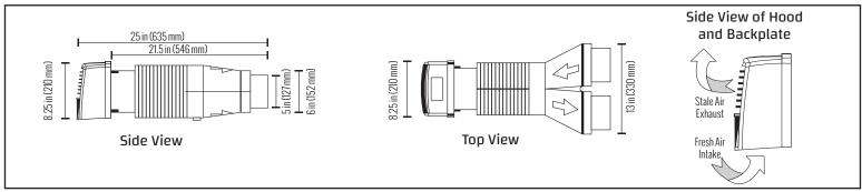
Figure 25. Dual Intake and Exhaust Hoods
