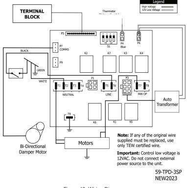
Figure 43. Wiring Diagram
